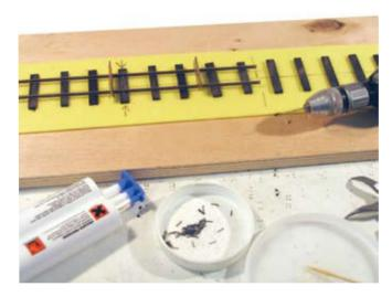
KBscale now produce roller gauges for O14 as well as the original RCL gauge. If locating rails adjacent to some already laid, then use small clamps or bulldog clips, to ensure the rails are in line (12). Mark each rail foot with a scriber in the centre of the feed sleeper and also press 2 points in the sleeper, exactly either side of each rail foot, at the feed location.
