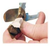
wander — possibly cutting just a few staples at a time, gradually moving the snips along the strip. Trying to cut corners by using long strips tends to produce long spikes at the end of the strip which will have to be discarded.
