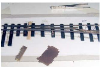
at the ends. Cut slots and fit power feed wires as before. Assemble the curved closure rail, switch rail, hinge and inside straight closure rail in the hinge soldering jig as before, then solder, file, polish and clean-up.
