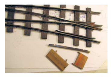
snug fit, file small nicks with a triangular needle file. Now blacken the check rails which ensures the rail ends are also blackened (20).
