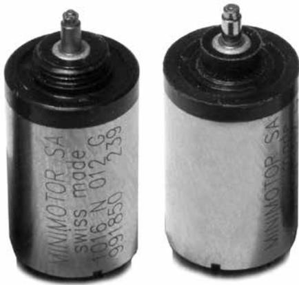
Left to right: Un-modified motor, motor with threaded 'nose' turned off, motor with new brass mounting and screws.
