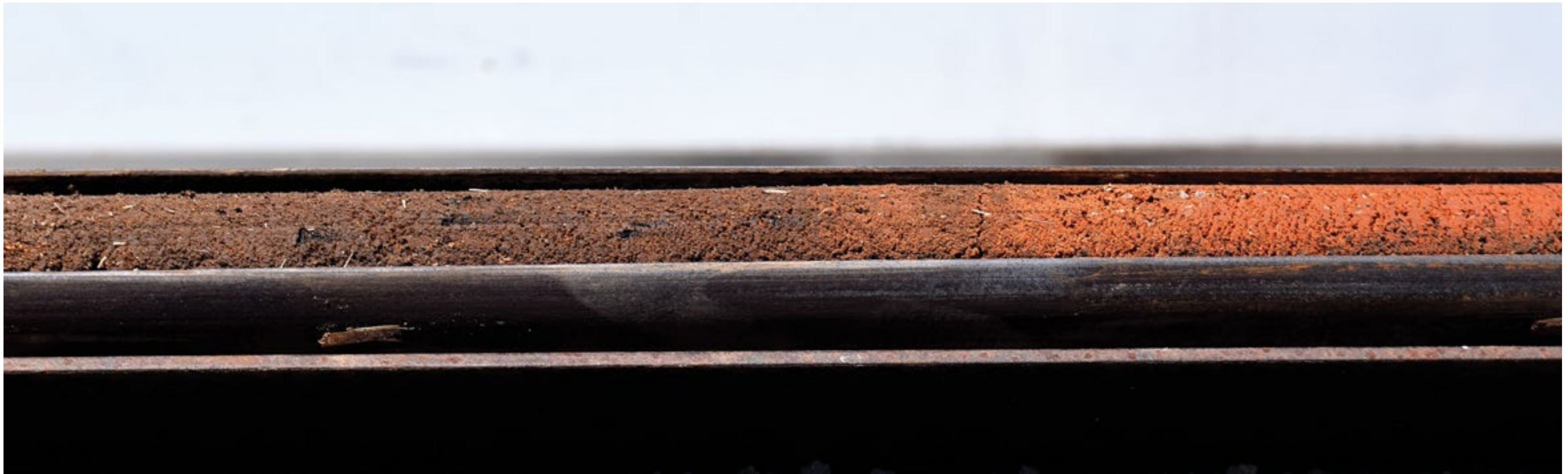
In this meter-deep soil core, the color changes from dark, organic matter-rich topsoil to red subsoil, where fewer roots have grown to add carbon.
