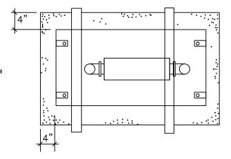
Step 1: New concrete installation you will need a couple of 2'x4' for resting the enclosure across the forms while the concrete sets up.
