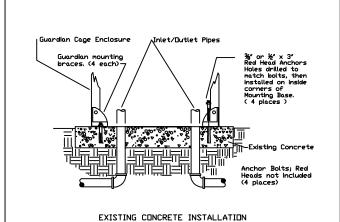
Using Mounting Base, set over existing backflow and center on concrete. Anchors will need to be drilled and set for the Moounting Base. Manufacturer recommends minimum of %x3' red head anchors to secure Base in four locations.
