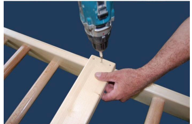
6. Use 3" screws to attach horizontal crossbars to vertical rails. Secure the unit to the wall with the lag bolts provided. Test the unit for stability before use.
