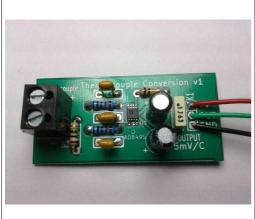
This **Thermocouple Amplifier Kit** is based upon the AD8495 precision K-type thermocouple amplifier. This can be used to measure very high temperatures, with a range up to 1000C (depending upon the rating of the thermocouple). The output is a voltage equal to 5mV per degree with a linear scale. This makes it very easy to measure with an analog input to a microcontroller (such as the Arduino).
