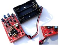
Battery cable goes through large hole then back in to PCB. Red: +ve Black: -ve
