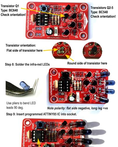
Double check IC orientation! Does notch align?
