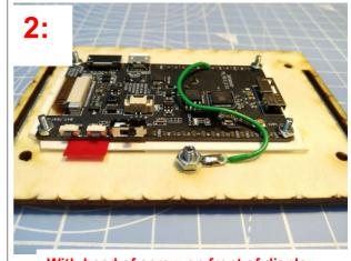
With head of screw on front of display, hold touch sensor solder pad, add Nut and tighten.
