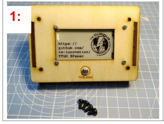
Align the front display section to the two slots. Ensure the display is the correct orientation.
