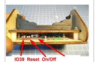
Pressing button "IO39" will put the unit into Access Point mode for updating configuration parameters or changing WiFi SSID and password.
