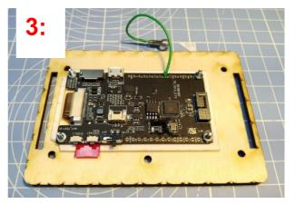
Align E-Ink board to four M2 screws. Check orientation of display (touch hole should be at the bottom). Add M2 nuts and tighten.
