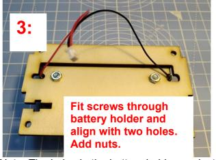
Note: The holes in the battery holder are just 3mm, so the screws might need turning to get them through the plastic holder.
