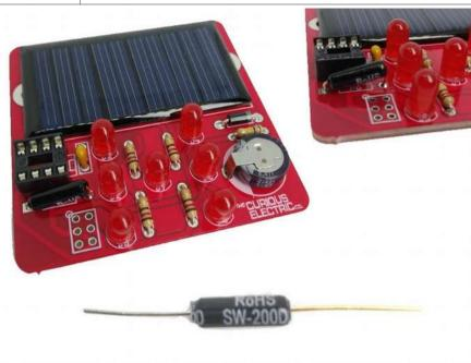
The vibration switch contains a small metal ball which connects some contacts to trigger the circuit.
