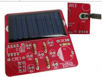
The solar panel must be soldered with the correct orientation.
