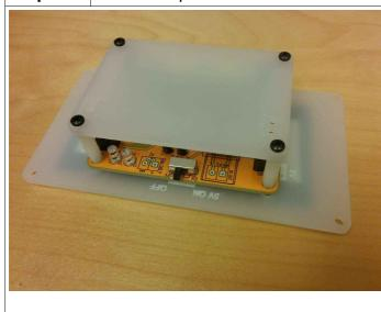
Use the 4 x M3 6mm screws to hold the back panel in place.
