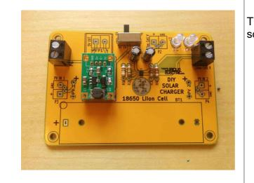
Then fit the DC-DC converter and solder this from the top of the board.
