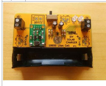
The IC is a surface mount device and almost impossible to solder by hand, hence we have already soldered this component for you.
