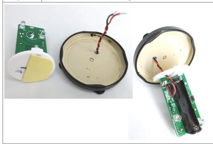
With the cable through the jam jar lid, solder the red +ve cable to the pad marked with a + on the 'Solar' connections.
