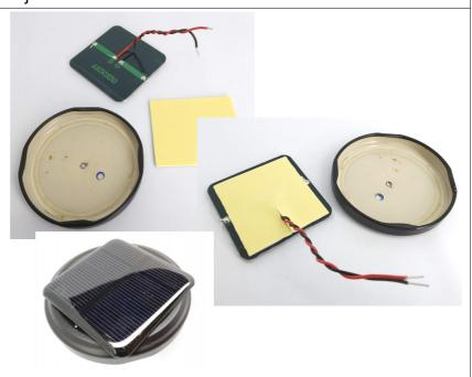
**Step: 9** Fit solar cell cable through and solder
