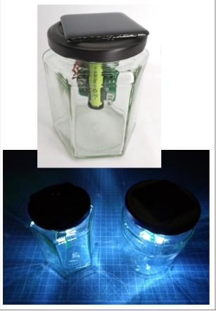
Convert an old jam jar into an outdoor solar powered night light!
