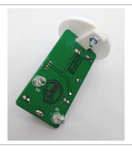
Put the two screws through the plastic, ensuring the screws go through and the heads are countersunk.
