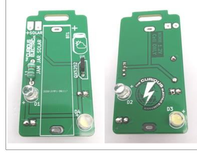
Insert LEDs D1 and D4 from the front of the PCB.
