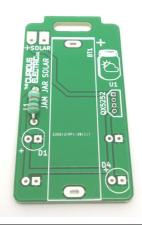
Place the inductor L1 into the holes on the PCB.
