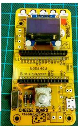
The OLED unit pushes into the 4 way header pins soldered in step 6.
