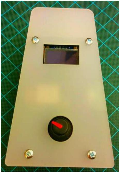
This is an ESP8266 breakout board with small OLED display, a rotary encoder for user input and five Red-Green-Blue WS2812 LEDs.
