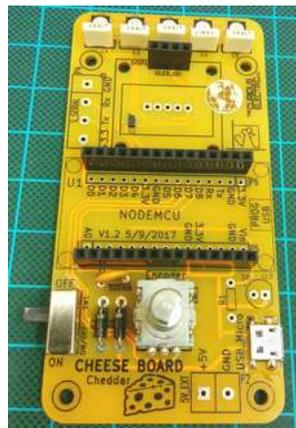
The encoder is soldered into the area marked ENC1.
