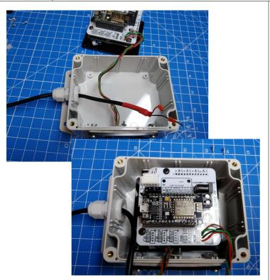
Put the USB power cable through the compression gland, with the power terminals through into the enclosure. It's easiest to add the USB lead now, or else it's more difficult with the sensor/baseplate in place.
