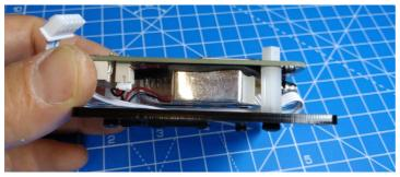
The SDS011 is mounted on the baseplate with the 20mm spacers towards the baseplate. The fan fits into the cut-out of the baseplate.
