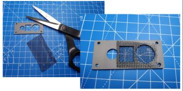
Cut the piece of mesh to a size that covers the larger round and the middle rectangular hole. **Step: 8** Add mesh, gasket and sensor plate
