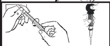
Figure 5: While centering spine plate, align with front u-bolts and mark skid plate for clearance hole drilling.
