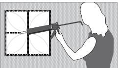
Installing with FRP Adhesive or Construction Adhesive, apply a thin bead of adhesive to the parimeter of the panel and smooth out with an adhesive spreader so adhesive doesn't seep out when pressed to the wall. Also apply a small amount on touch points in the center of the panel. Follow manufacturer's recommendations on dry times.
