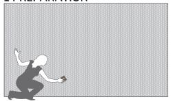
Install over primered or painted drywall or plywood. Surface must be clean, smooth, dry, free of waxes and existing adhesive, dirt, dust, grease, oil, paint curing compound or sealers.
