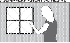
If choosing to install using the Harmony Peel + Stick Tape, apply the tape to the perimeter plus strips across the panel on the touchpoints. Each corner should be covered. Press tape firmly to the panel. Peel backing off and adhere with pressure.
