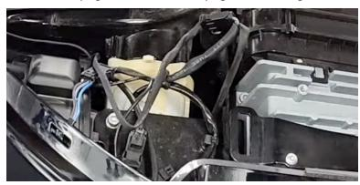
• Re-Install the plastic cover with a little over an inch of slack on the outside of the plastic cover.
