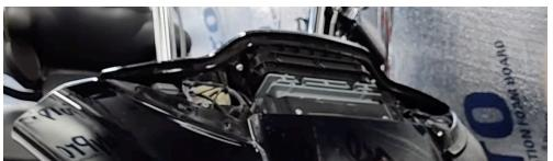
• Locate the turn signal plugs under the fairing. There will be one of the left and one on the right.
