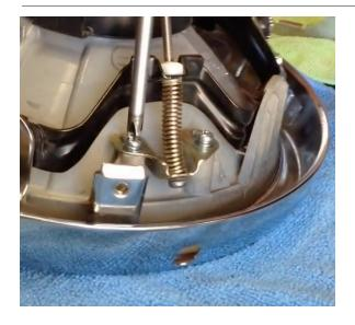
Now the reflector housing can be removed from the mount. It should lift directly off of the reflector.
