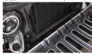
**Step 8: Reinstall the top clips.**Reinstall the top clips to the grill. Push the clip down to relock it. Repeat for all 6 clips.
