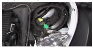
Step 5: Connect the LED Headlight Install the new headlight into your Jeep utilizing the harnesses in the kit.
