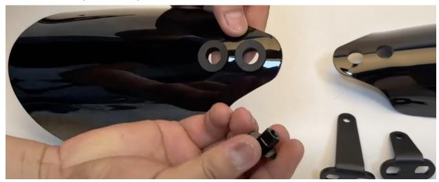
• Install the bracket on the handshield using the and provided hardware.
