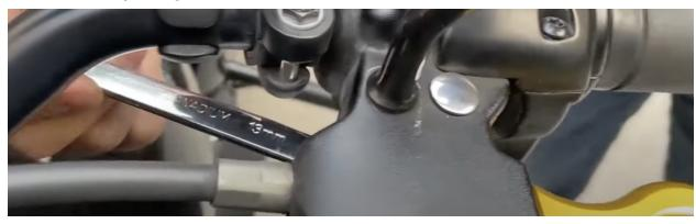
• Install onto the bottom of the mirror stem. Use original hardware to secure it to the bike.
