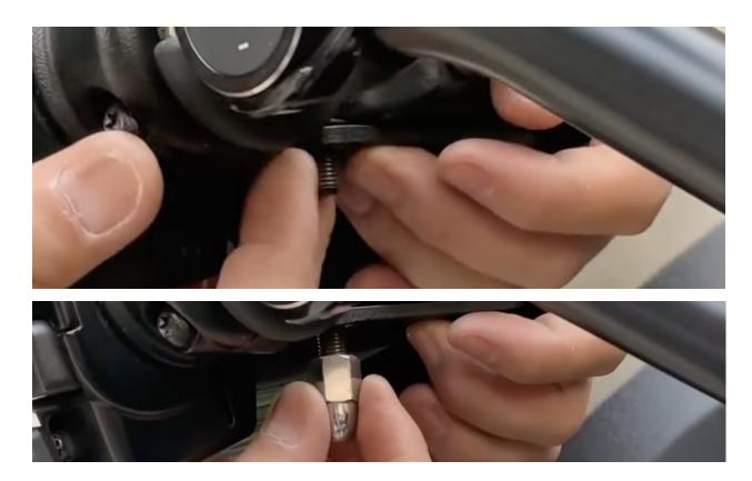
• Tighten down the nut and make sure it does not move.
