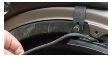
• Remove the wire retainer that holds the wiring harness.
