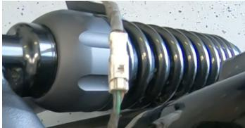
• Starting with the left (clutch side), remove the strut brace from the bike by using a 5mm allen key.
