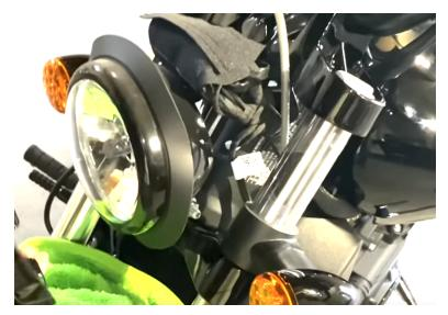
Remove screws on either side of the headlight.
