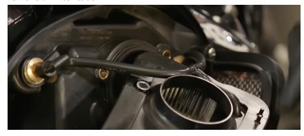
4. Remove original air filter backing
