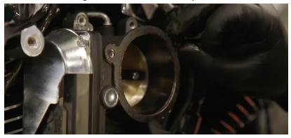
7. Place gaskets onto bolt holes on either side of the new air filter backing plate.
