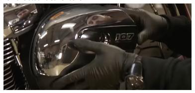
2. Remove the stock air filter. Remove any bolts holding in the air filter.
