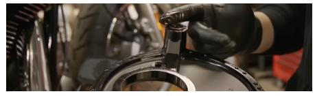
8. Install backing plate on the throttle body with provided bolts.
