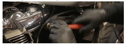
5. Remove original air filter bracket
