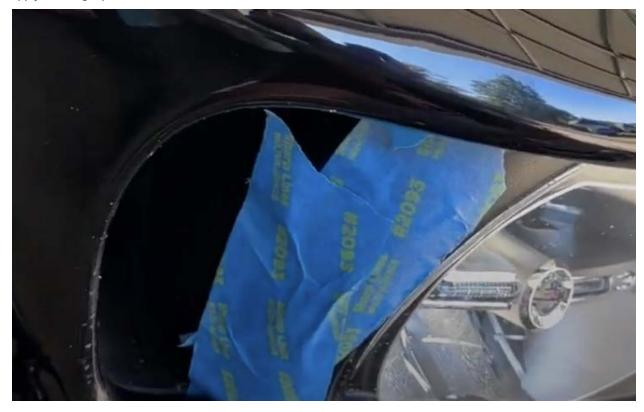
9. Align the turn signal in the vent.
