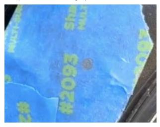
11. Drill with a 5/16 drill bit on both top and bottom.
