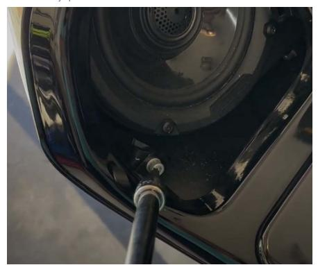
5. Remove bottom screw on the fairing. Do this on both sides.
