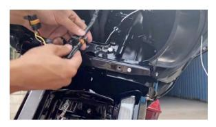
Disconnect the turn signal wiring. Leave disconnected for now
