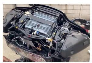
Remove screws holding in the headlight. Unplug the headlight and place it to the side. Remove side bolt.
