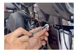
Route the wiring from the fork LED light up into the space for the headlight.
