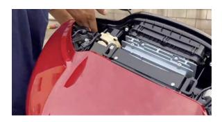
Remove the bolts holding on the fairing and the bolts to the turn signal bracket.
