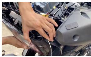
Connect the turn signals from the fork turn signal to the turn signal wiring on the bike.
