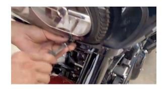
Place foam on the inside of the new fork LED light. Align on to the forks. Using the bolt removed from the previous step, attach the fork LED light to the bike.
