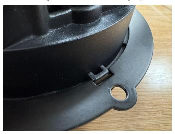
d. Use the final trim ring to hold the headlight into the motorcycle. (Note: The picture below shows the headlight not installed on the motorcycle.)
