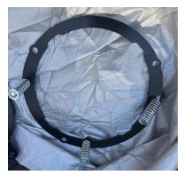
d. Detach the cradle ring from the mounting ring by removing the three bolts with springs. The cradle ring, bolts and springs can be discarded.
