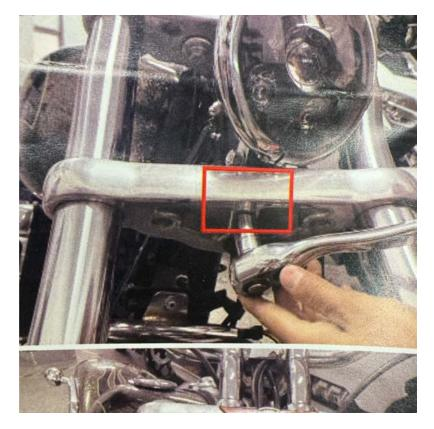
• Undo the two bolts underneath the handlebars. The bracket will connect with these bolts. As shown below:
