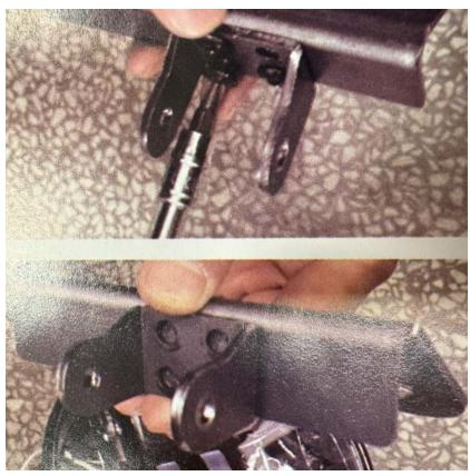
• Remove the seat and the bolt below the fuel tank. The bolt does not have to be completely undone. You will find the original headlight plug there. Disconnect the plug as shown below:
