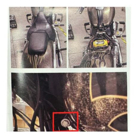
• Unbolt the original headlight. The bolt is located on the bottom of the triple tree as seen in the picture below:
