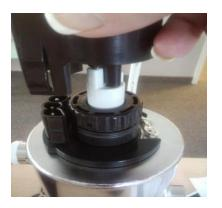
Attach the lamp to the lamp harness and lower the lamp into the chamber.
