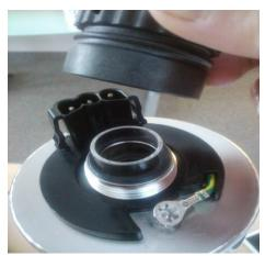
Remove the lamp connector base from the lamp harness on the BA-ICE-S. Remove the sleeve bolt and place the ring adapter on the chamber. Secure the ground wire to the chamber.
