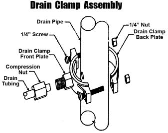
NOTE: Some local laws and regulations require the use of an air gap faucet. To assure compliance check your local plumbing code. Locate the drain connection away from the garbage disposal to prevent potential contamination and system fouling.
