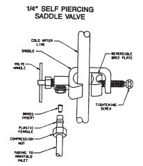
Do not over tighten the clamp. The clamp should be secure and resist a slight twisting force. Turn the saddletapping valve clockwise until the needle fully pierces the tubing and the valve seats. For maximum flow, back the handle out all the way. Adjust as required.
