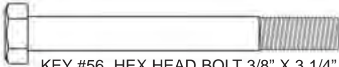
KEY #56 HEX HEAD BOLT 3/8" X 3 1/4" PARTIAL THREAD QTY. 2
