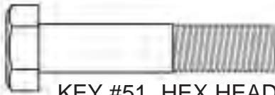
KEY #51 HEX HEAD BOLT 3/8" X 1 3/4" PARTIAL THREAD QTY. 22
