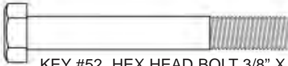
KEY #52 HEX HEAD BOLT 3/8" X 2 3/4" PARTIAL THREAD QTY. 4
