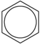
PART # 56 HEX HEAD BOLT M10X90L PARTIAL THREAD QTY.1
