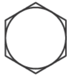
PART # 51 HEX HEAD BOLT M10X50L PARTIAL THREAD QTY.1
