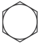
PART # 50 HEX HEAD BOLT M10X45L PARTIAL THREAD QTY.18
