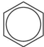
PART # 52 HEX HEAD BOLT M10X55L PARTIAL THREAD QTY.2
