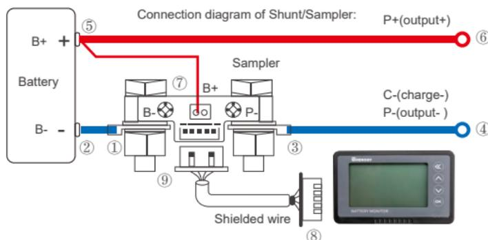
Attention: Please connect as shown. The shunt must be series connected to the negative circuit, DO NOT connect to the positive circuit.
