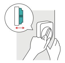
Remove the battery insulation tab by pulling it away from Sesame.
