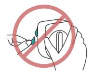
Never pull the adhesive strip toward you as this will cause the strip to break. Always pull the strip parallel to the door. If there is leftover adhesive on your door, you can use floss to scrape off the remaining pieces without damaging your door.
