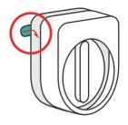
Tuck the adhesive strip back under the cover when replacing the cover.
