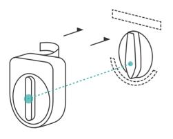
Remove the backing of the adhesive strips and attach Sesame to your door. Be sure to line up the axes of rotation of Sesame and your lock during installation for best results.
