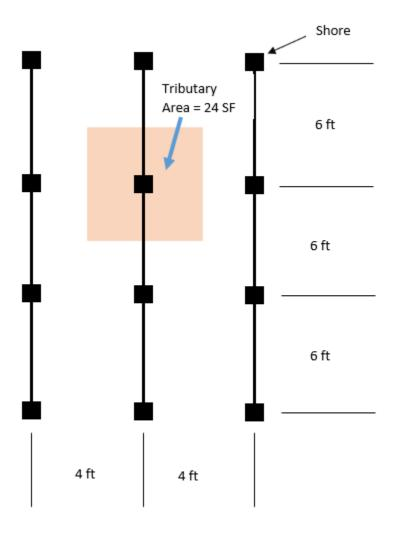
Therefore, the load carried by an individual shoring member in this illustration would be 24 square feet (i.e., its tributary area) multiplied by the load (formwork, concrete, construction, etc.) from above. The formula is simply:
