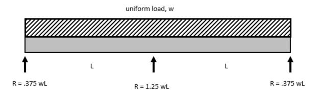
In this condition, the reaction of 1.25wL in the middle would mean the shore at the interior support would theoretically support 25% more load than the "simply supported" case. For simplicity, the discussion herein will not use any continuity factors but the construction management student should be aware of what they are and why they might be used in shoring system design.
