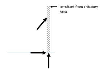
The brace acts as a two-force member with the "reaction" force acting in the direction of the brace.
