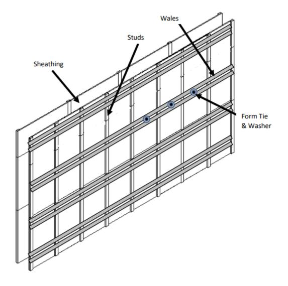
Previously we discussed wall forms that were subjected to wind loading prior to concrete placement. Now we are interested in understanding wall form performance with concrete placed inside the form. When concrete is placed into the wall forms it produced a lateral pressure that can be quite high. In order for the finished walls to be of high quality, the formwork has to be stiff enough and strong enough so that the
