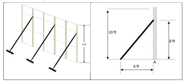
It is typically assumed that one-half the wind load gets distributed to the top and the other onehalf is distributed to the bottom of the form. The area of wall form that distributes to the top is:
