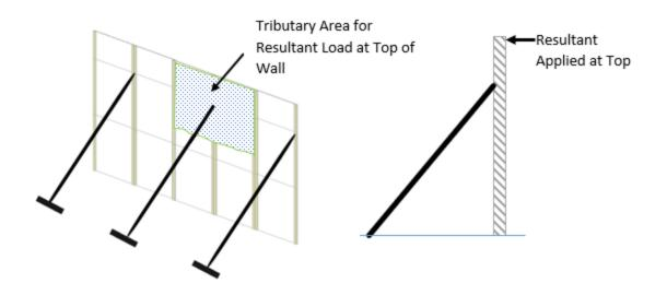
The determination of the load that must be carried by one brace follows the principles of equilibrium which were discussed earlier in this text. In this case the wall form acts as a beam (oriented vertically) and it can be assumed that the brace acts as a "link support" and the bottom of the wall form is pinned. So, the free body diagram would look like this:
