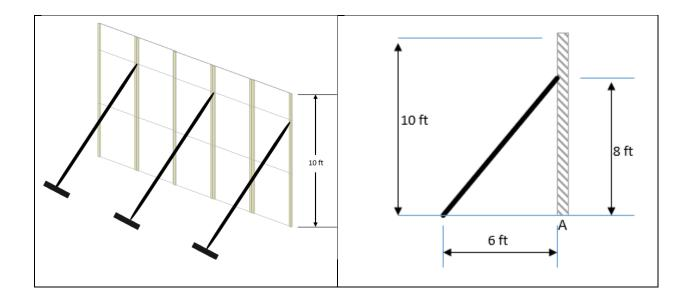
In this case, if the brace can carry 2000 lb, then based on its geometry the x-component could carry (6/10) (2000 lb) = 1200 lb.
