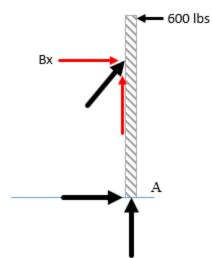
Summing Moments about point A will solve for the horizontal bracing component (i.e., the horizontal red arrow called Bx) as such:
