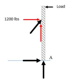
Summing Moments about point A will solve for the horizontal bracing component (i.e., the horizontal red arrow called Bx) as such:
