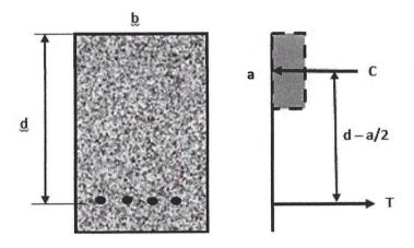
The "d" distance shown stretched from the compression side of the beam to the centroid of the steel (where the T force acts). The "d" distance is sometimes referred to as the design depth or the effective depth. Therefore, the nominal moment capacity of a beam is given by the following equation:
