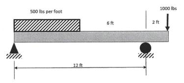
To begin with, the support reactions must be solved correctly (refer back to the earlier section if you need guidance on equilibrium equations – it is imperative that you get the reactions correct!). The reaction are as shown below.
