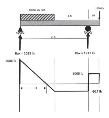
The "x" distance where shear would be zero is?
