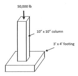
The stress in the column and the stress under the footing are both compressive stresses, although technically we refer to the stress in the soil under the footing as a "bearing" stress. Both of these stresses will be calculated by the following formula:
