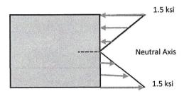
If a beam is not symmetrical, then its neutral axis will not lie "in the middle" of the shape and therefore this will result in a "c" value for the top of the beam and another "c" value for the bottom of the beam. Of course, the different "c" values will result in different bending stresses at the top outside edge and the bottom outside edge. The following example will demonstrate this concept.
