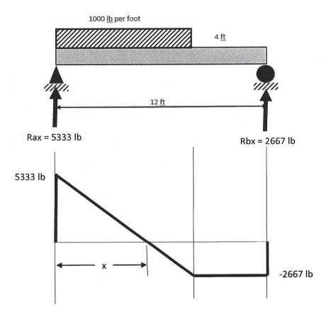
One item to determine is where the diagonal line of the shear diagram crosses zero. The diagonal line is a straight line with a slope of -1000 lbs per foot so the "x" distance is simply calculated as:
