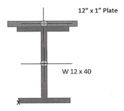
Filling out the table with a, x, and y values we can then sum the "a", "ax" and "ay" columns and calculate the  $\bar{x}$  and  $\bar{y}$  formulas as shown below.
