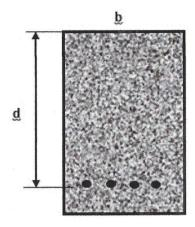
Starting out, calculate the resultant tensile force, T.
