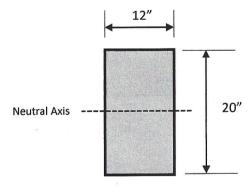
Rectangular shapes have a moment of inertia that can be calculated from the formula:
