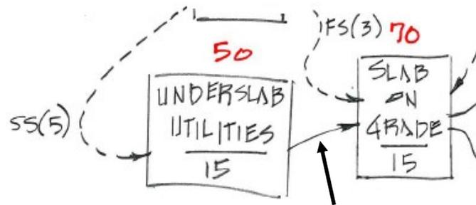
1. First off, from the partial hand-drawn schedule above, you can see that the relationship between the **Underslab Utilities** activity to the **Slab on Grade** activity is a finish to start relationship with no lag.
