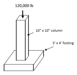
The footing size has to be redesigned because the actual stress (10,000 psf is greater than what is allowed 2500 psf). So the 3 ft. x 4 ft. footing size has to be increased. We can perform a redesign using the following formula but re-arranging it:
