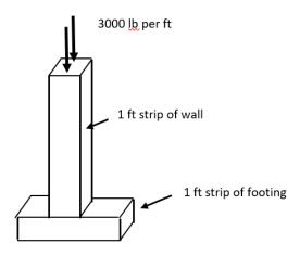
The total load on the 1-foot strip is 4500 pounds per foot (i.e. 3000 +1500). The area of the continuous footing over a 1-foot strip would be:
