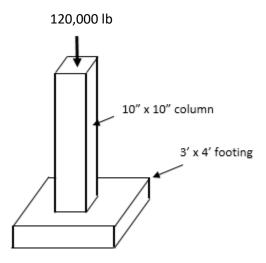
The stress felt by the soil under the footing is a bearing stress and is calculated by the following formula:
