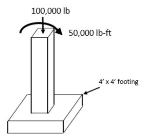
The maximum bearing stress will occur on the "right" side of the footing while the minimum bearing stress will occur on the "left" side. The stress is always maximum of the side where the moment is "pointing". Compressive stresses will be assigned a "negative" sign. The formulas to be used are as follows:
