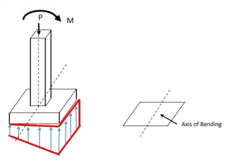
This "combined" bearing stress is a combination of the direct compressive stress,  $\frac{P}{A}$ , and the bending stress caused by the moment M (remember bending stress is equal to  $\frac{M c}{I}$ ). If we assign stresses that create compression a negative sign and stresses that cause tension a positive sign, then the maximum and minimum bearing stresses are as follows:
