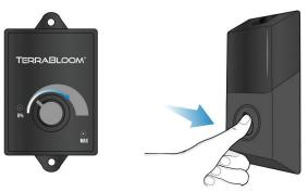
• To prepare fan for operation, attach your preferred speed controller to the fan before power on.
