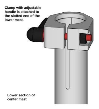
The clamp handle can be set in any position once the clamp is tightened pull the handle out slightly and turn to a suitable position.
