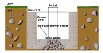
Place some small stones in the bottom of the hole, just under the bottom end of the socket and surround them with cement, this will allow rainwater to drain away.
