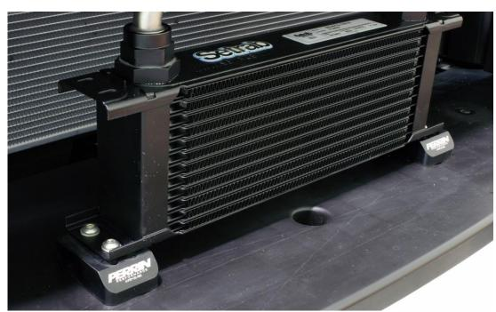
15. Install supplied M6 washer onto M6x65 bolt. Then install 1.25"OD washer onto M6x65 bolt. Install bolt with washers from bottom of car up through splashguard into PERRIN Oil Cooler Brackets. Tighten bolts down to roughly 15ft-lbs or just beyond hand tight. **NOTE: Do not over tighten these bolts, as they will eventually break through plastic part of splashguard.**
