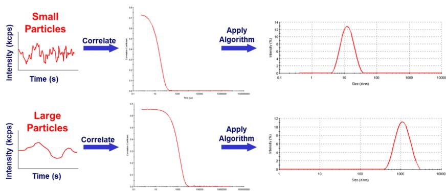
Figure 2. Correlation of Intensity Fluctuation to Size Distribution by DLS
