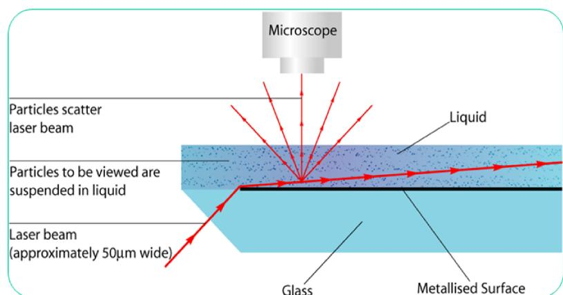
Figure 1. Schematic of the optical configuration used in NTA
