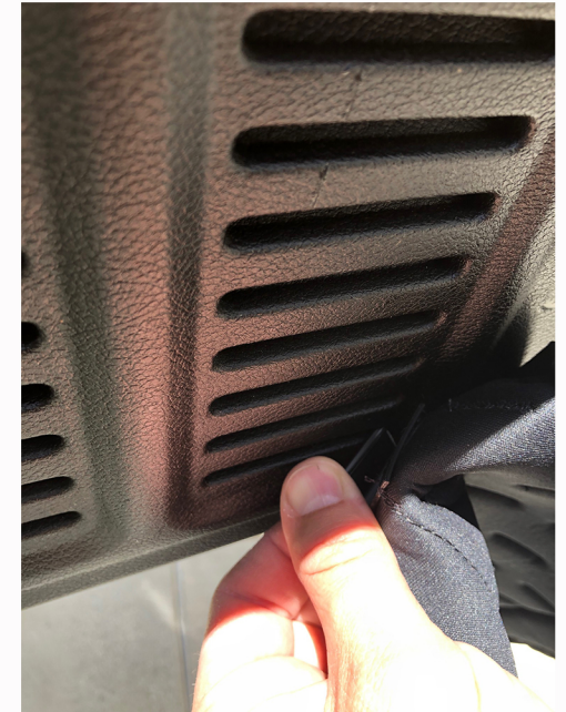
3) Starting with the left or right side, insert all 4 plastic tabs into the bottom slot they line up with
