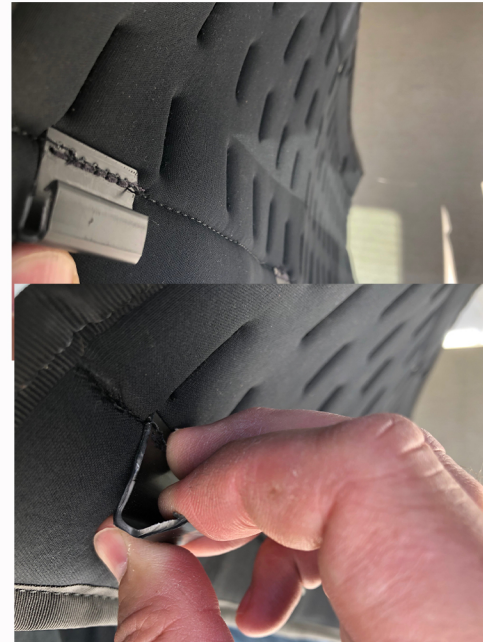
2) At the bottom of the Bartact panel pull the plastic tabs to open them slightly wider
