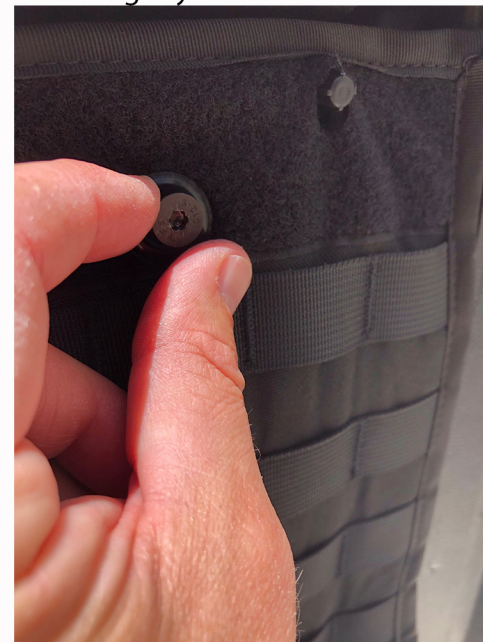
5) Finger tighten the 3 included torx bolts, and then finish tightening them with a torx bit
