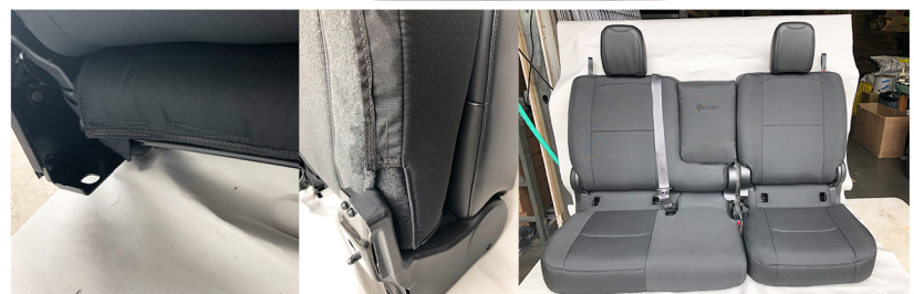
Install the smaller section in a similar fashion, and you are ready to go after reattaching the center seat belt
