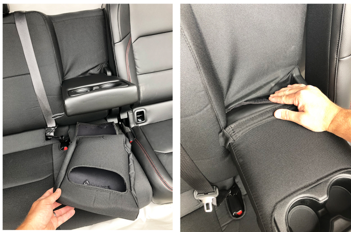
Fold down the armrest and slide over the armrest cover. Then slide the velcro piece from the armrest cover though the bottom and attach both pieces at the top.
