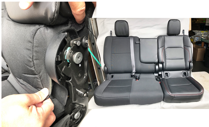
Secure the inside edge between the 60 & 40 sections of the bench as shown
