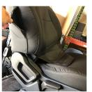
III) Slide the Top on the seat, making sure it is centered. (Check again to make sure the air bag opening is facing the outside of the Bronco). Push the bottom front of the seat cover through the back of the seat. Pull back tightly, especially towards the outsides of the seat, and secure the hook and loop between the front and back sections until it is snug.
