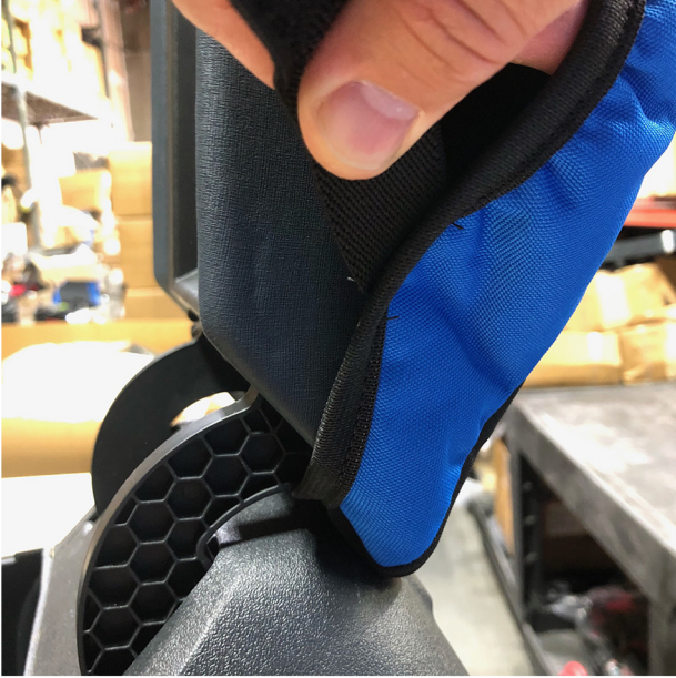
1) Detach velcro straps and slide the back of the cover over the rear corners of the console lid
