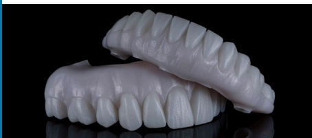
Above: Sintered after infiltration – Zirconia hybrids infiltrated in green state, then sintered according to manufacturer instructions. Photo and case by Vadim Vainer, Shiksha Dental Laboratory.
