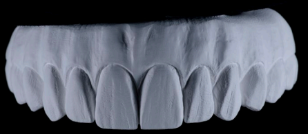
Above: First stage of green state – Initial refining of milled green state zirconia. Photo and case by Vadim Vainer, Shiksha Dental Laboratory.
