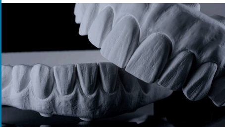
Above: Second stage of green state – Final contouring and texturing of green state zirconia. Photo and case by Vadim Vainer, Shiksha Dental Laboratory.
