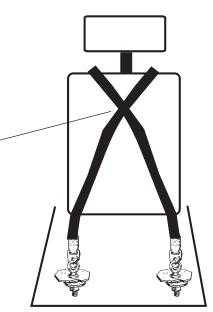
(View behind seat showing the floor anchor mounts)
