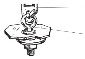
Rear part of shoulder-harness portion of seatbelt kit (belt ends connect to the included Grade 5 eye bolt or to your harness bar or roll bar system)
