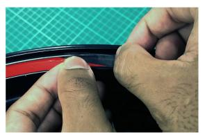
Align Protect sticker to cover total area of sharp edge of outer rim strip attached to rim.
