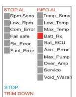
"Temp\_Sens" indicates a temperature probe failure
