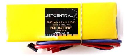
Jet Central supplies and recommend 9.9v 3s LiFePo batteries, however 11.1v 3s LiPo may be used. Important Note: if you have to make extension wires for the battery, make sure to use quality wire and follow these gage wire suggestions: up to 40cm (16") use 14 AWG, from 40cm to 80cm (16" to 32") use 12 AWG, and from 80cm to 150cm (32" to 60") use 10 AWG
