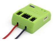
The 3Digi HC variant (HC = high current) has 2 additional cable for direct connection of the external power. These cables have a sufficiently large cross section so that there is almost no loss of voltage between BEC and 3Digi even with power-hungry servos. The cables can be fitted out with various plugs or sockets. We recommend, for example, 2mm or 3,5mm gold contact plugs.
