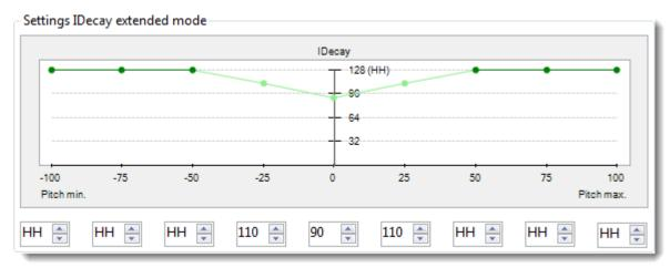
If the value "Extended" is selected in the combo box *IDecayMode*, the values here will be enabled and you can make changes here.
